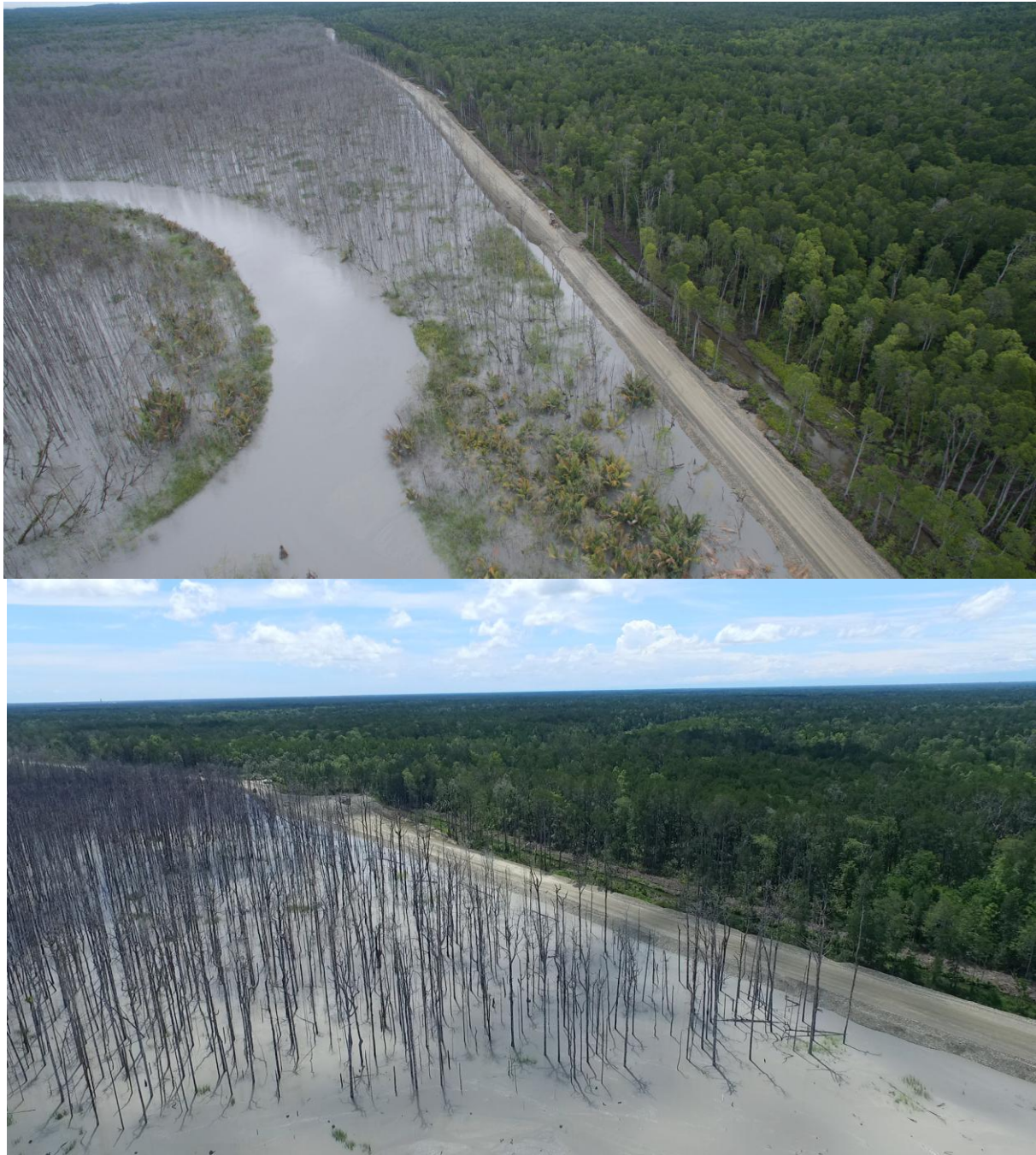
Withered trees in tailings slurry deposition area, and green trees outside of the deposition area, separated by a dyke.
